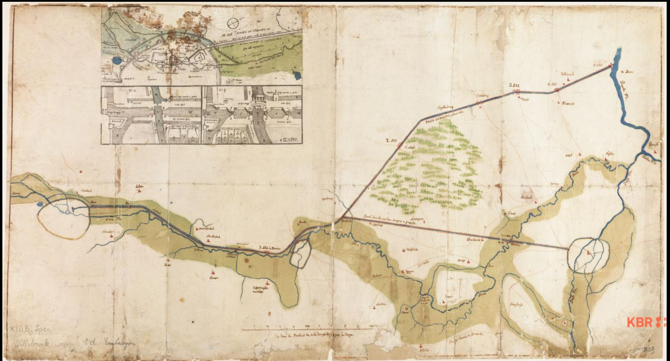
Michiel van Langren, Proposal for an extension of the Brussels navigation towards Mechelen , 1663. Pen and ink on paper with an engraved inset showing a system of locks and sluices outside of Brussels, 23.5 x 39.5 cm Brussels, Royal Library
